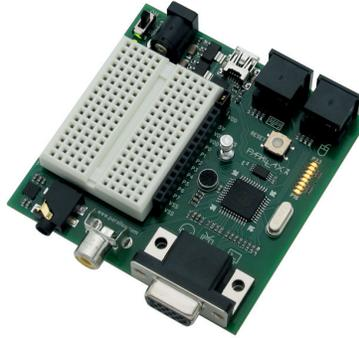
Figure 6: Parallax Propeller Demo Board
